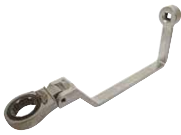
DA6119 Crows foot oil filter wrench Freelander 2 Range Rover Evoque 2.2 diesel 27mm x 1/2" D with switchable bi-hex ratchet head. Euro 6 compliant engines from 2010 onwards. Chrome plated chrome vanadium. Equivalent to OEM 303-1579
