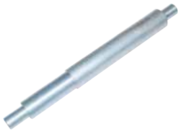
DA1147 Clutch alignment tool Defender - 2007 onwards Discovery 3 - TdV6 manual Replace two tools for one with this cost effective clutch tool. One end is the Land Rover 308-419 clutch alignment tool which is used to align the clutch disc and pressure plate on installation. The other end of the tool is Land Rover 303-1096 aligner/installer tool which is used to align the clutch drive plate and install the spigot bearing.
