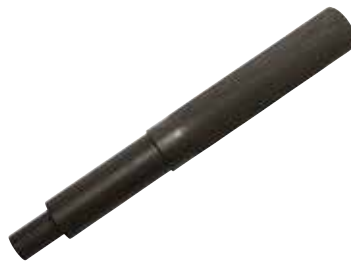
DA6113 Clutch alignment tool Defender - 2.4 TD4 - 2007 onwards Specifically designed to hold the clutch centre plate centred on the flywheel while fitting the clutch cover plate. Ensures fast effective alignment of the clutch centre plate. 200mm long x 14mm dia with knurled grip. Equivalent to OEM 308-419.
