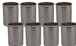
DA1185 This flanged repair liner is suitable for damaged/porous 3.9/4.0/4.2/4.6 Rover V8 blocks. The block will require re-boring and flange recess machining before fitting. This liner is the complete solution for fixing these blocks. The liner can be bored to 96.00mm for over-bored versions of the V8 engine, taking it to 5.0 litres. Semi finished bore 94.00mm (less 1.00mm for final finishing in bore). Dimensions Inside diameter - 94.00mm; outside diameter - 99.06mm; length - 135.64mm; flange - diameter - 105.23mm; flange depth - 5.33mm
