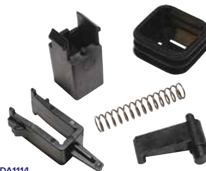
DA1114 Discovery 3/Discovery 4/Range Rover Sport - 2015 - 2013 This handy little OEM kit is used to repair the temperamental fuel latch.
