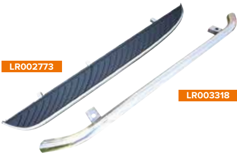
LR002773 Side step Pair Thermo plastic elastomer side step top and a brushed aluminium side trim. LR003318 Side protection tubes Pair Stainless steel
