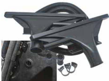
DA1205 Defender - up to 2007 Fitting this Defender demister kit will help demist your windscreen better than the standard fitted demister and has the added bonus that it will also demist your side windows too. With full fitting instructions.
