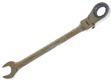
DA1189 For removing and installing oil filters on diesel models of the Freelander 2 and Range Rover Evoque. 27mm combination spanner with flexi head. 400mm long. Manufactured from Chrome Vanadium. Fully polished with ratchet. Manufactured to Ansi standards.
